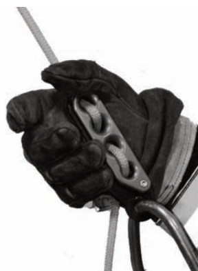
Squeeze lever to begin descent, with brake hand on the free end of rope.
