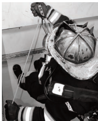
Once device is loaded, both hands are needed for operation: brake hand must be on free end of rope. Descent is controlled by squeezing release lever and varying pressure on free end of rope with brake hand.
